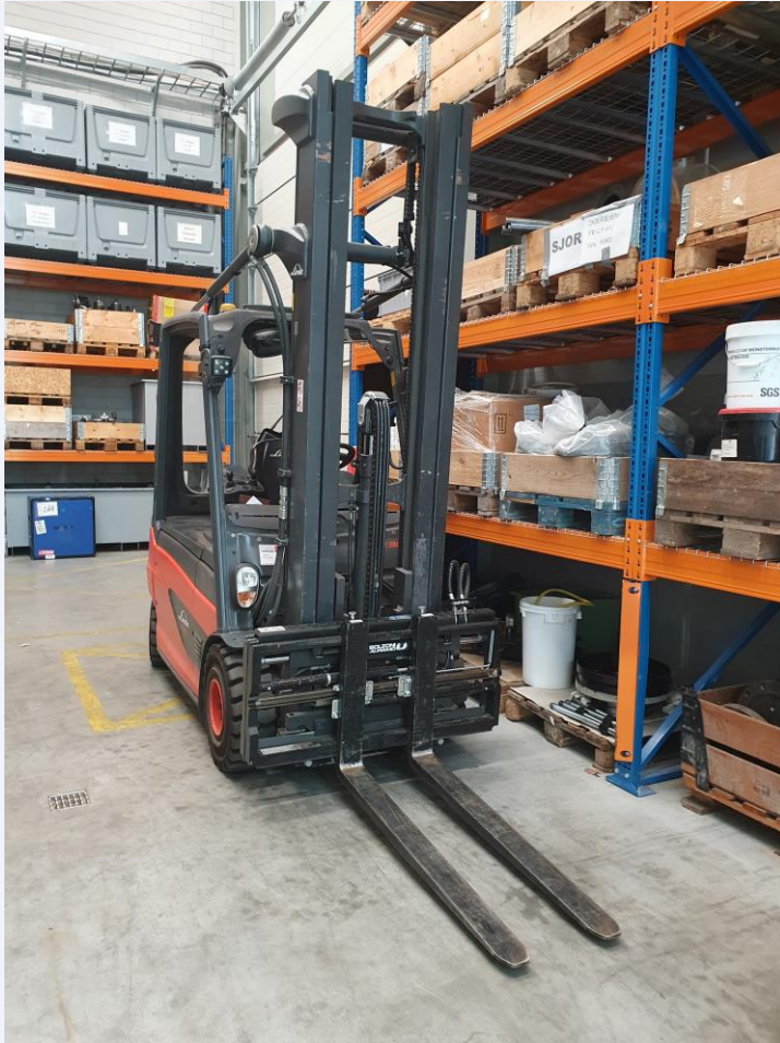
Forklift truck Linde Material Handling E30L-01 Max load 3000kg
